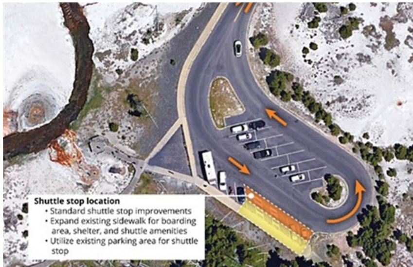
Figure A-1: Conceptual example of a ‘medium’ investment transit stop, at Black Sand Basin parking area
