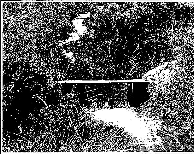
One of the weirs in the Boundary Creek area of Yellowstone that was equipped with electronic monitoring devices to store information on chloride flux that could be retrieved every few months.
