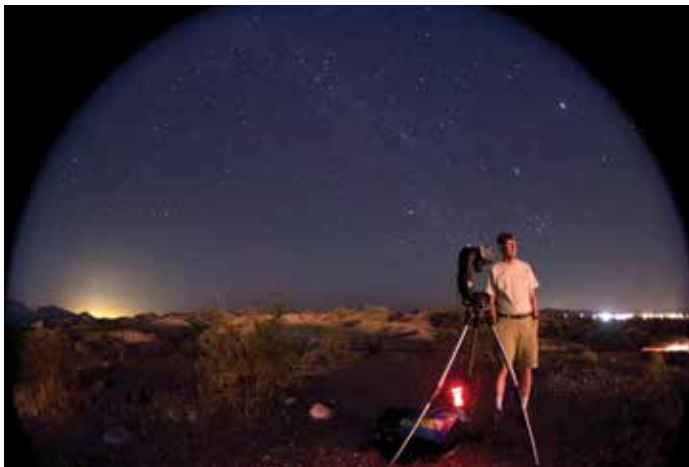
Using special camera equipment, an NPS scientist measures the brightness of light from outdoor and celestial sources across the entire night sky. Photo: NPS
