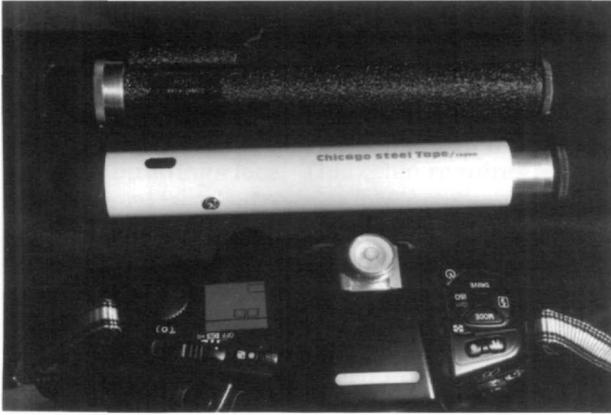
*Three levels. The top two are hand levels and the bottom is a bubble level mounted on the camera hot shoe. (Jeff Dean, 1996)*
