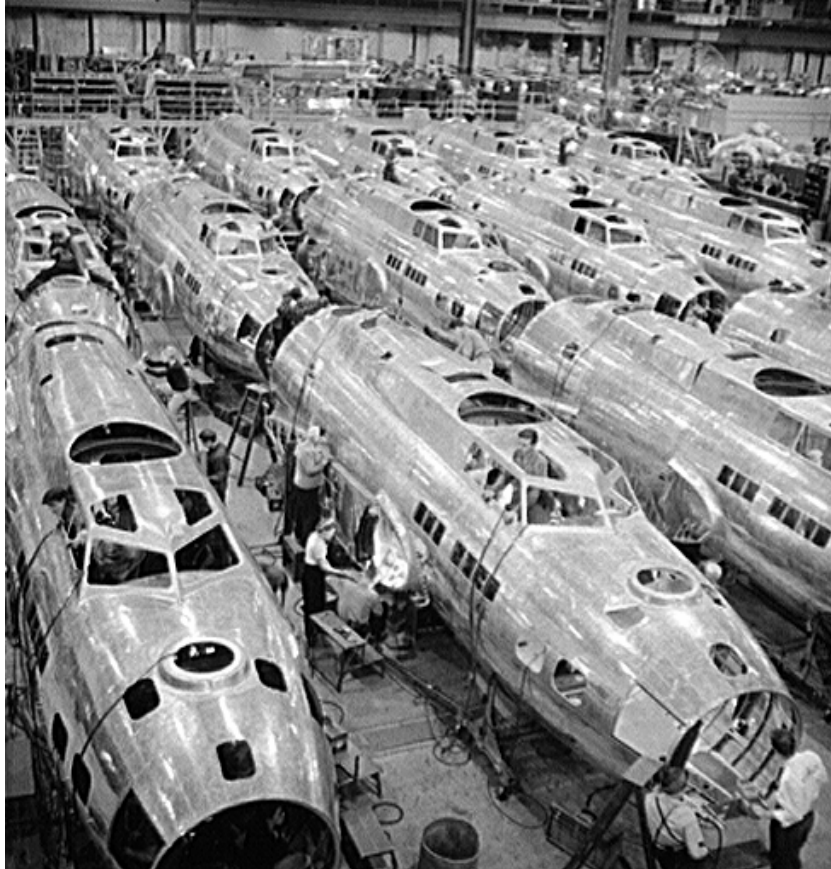
Workers at the Boeing Aircraft Plant in Seattle produced B-17F (Flying Fortress) fuselage sections. December 1942. Library of Congress, Prints & Photographs Division, FSA/OWI Collection [LC-USW3-041070-E].
