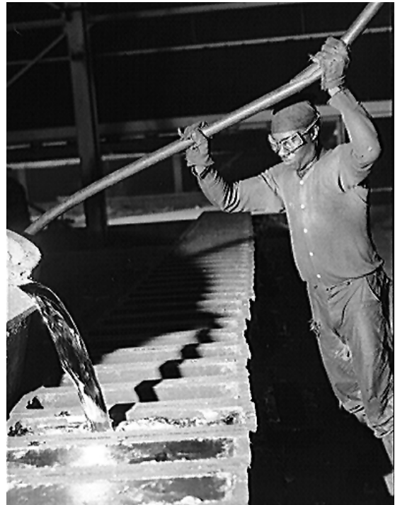
A workman pours aluminum into molds at the Reynolds Metal Company in Sheffield, Alabama. Possibly dates to August 1942. Library of Congress, Prints & Photographs Division, FSA/OWI Collection [LC-USW3-005438-D].
