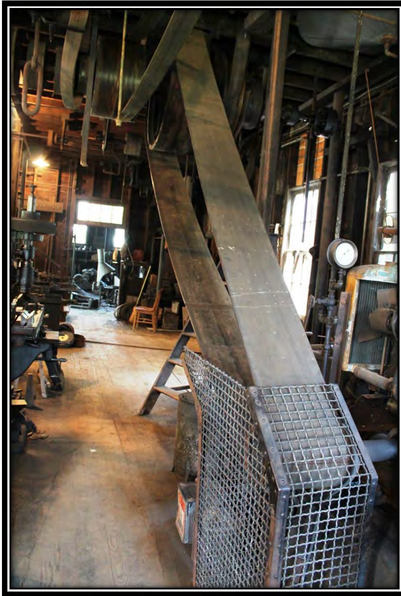
Photograph 15. PA_Greene County_W.A. Young & Sons Foundry and Machine Shop_0015. Main belt driving the horizontal line shaft, facing southeast.
