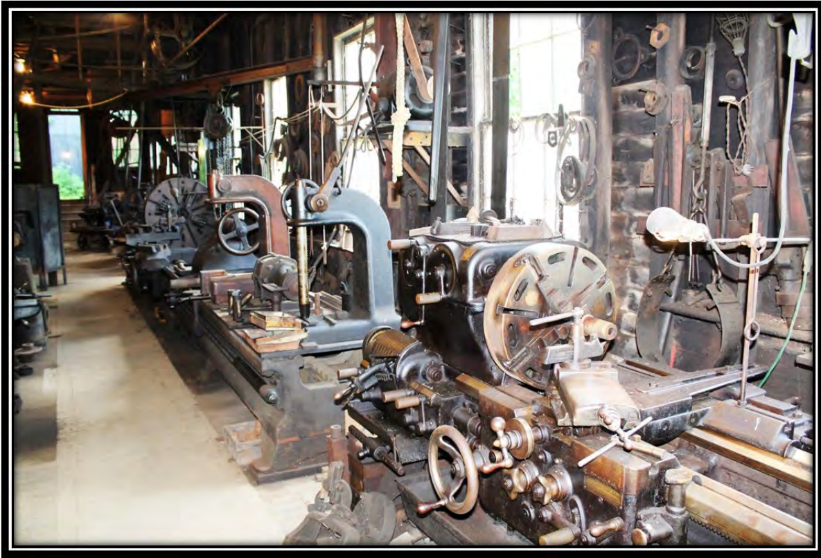
Photograph 18. PA_Greene County_W.A. Young & Sons Foundry and Machine Shop_0018. Engine lathes, shop-built broaching press, and electric grinder, facing southwest.
