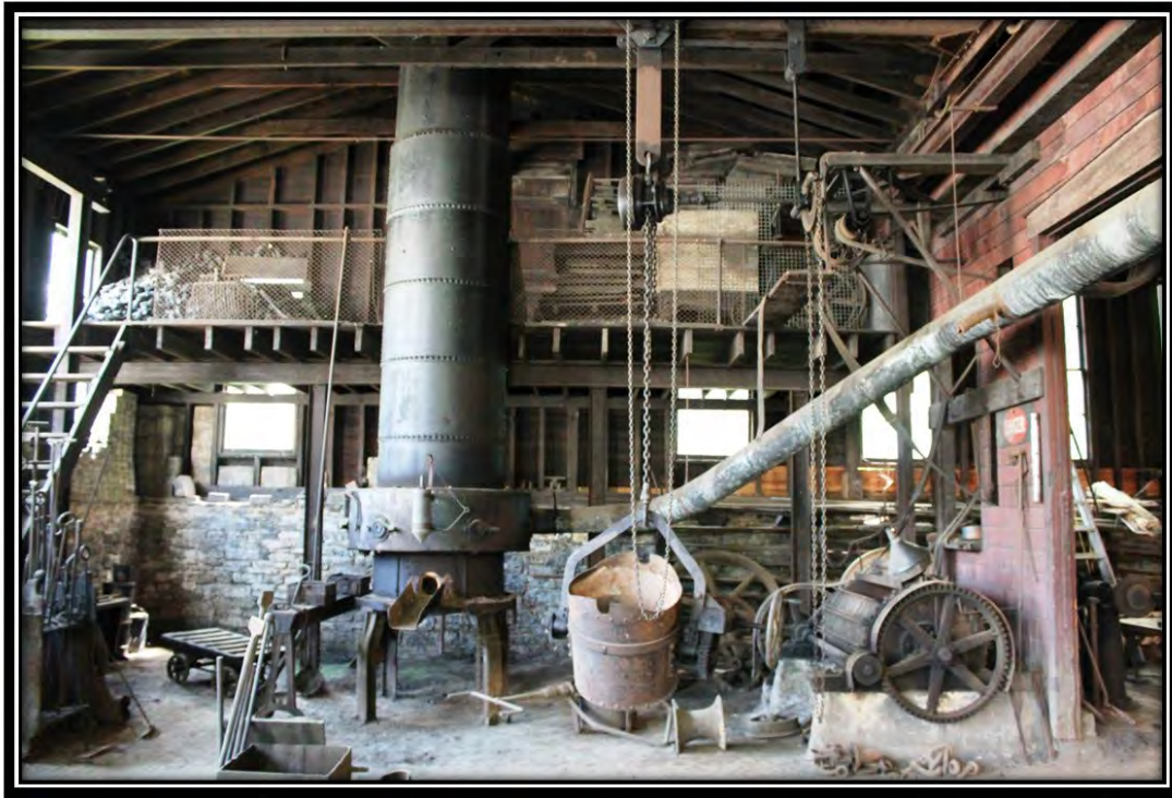
Photograph 33. PA_Greene County_W.A. Young & Sons Foundry and Machine Shop_0033. Cupola loft, cupola furnace, ladle, tuyere, and casting tumbler, facing southwest.
