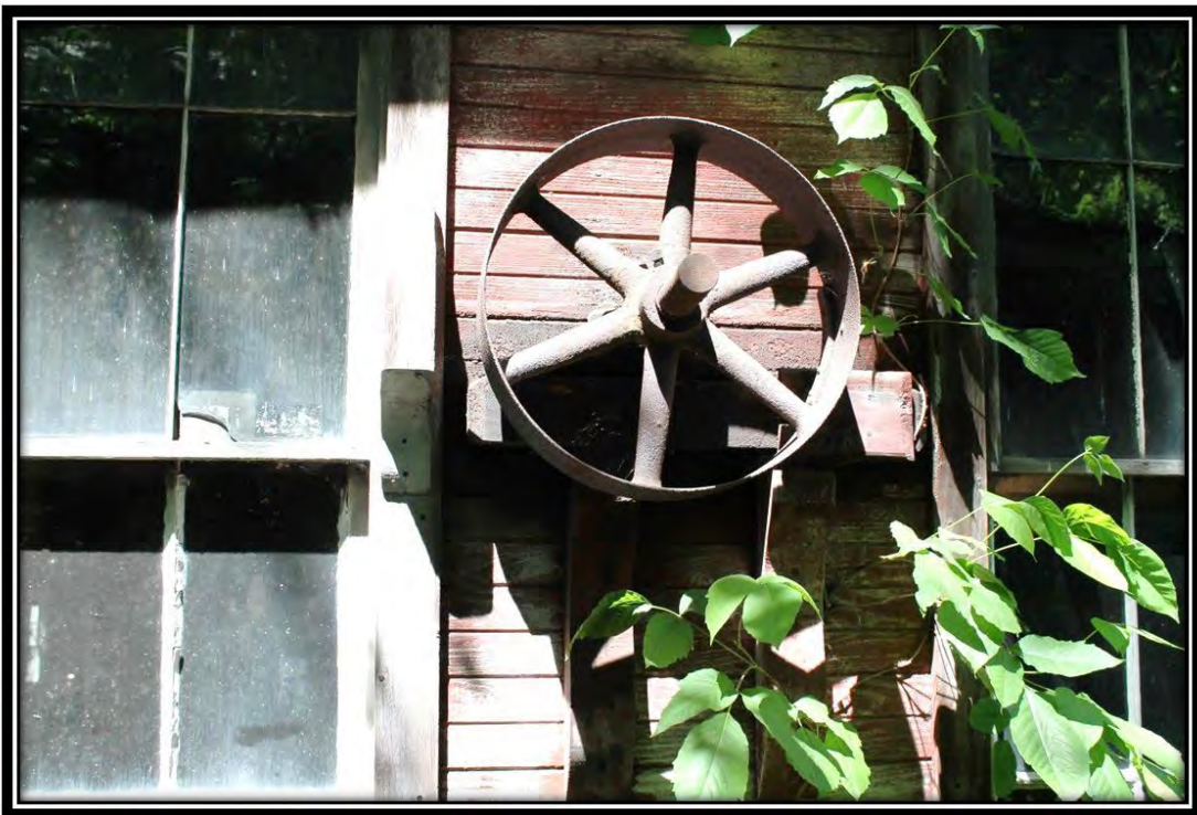
Photograph 10. PA_Greene County_W.A. Young & Sons Foundry and Machine Shop_0010. Flat-belt pulley on exterior of the line shaft at the back of the Rear Shop, facing northeast.
