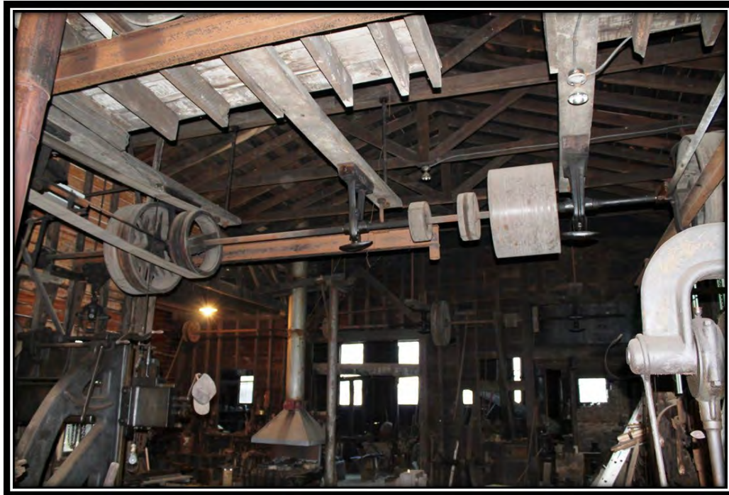
Photograph 13. PA_Greene County_W.A. Young & Sons Foundry and Machine Shop_0013. Horizontal line shaft in the Back Shop, facing east. In the background is a hand forge.
