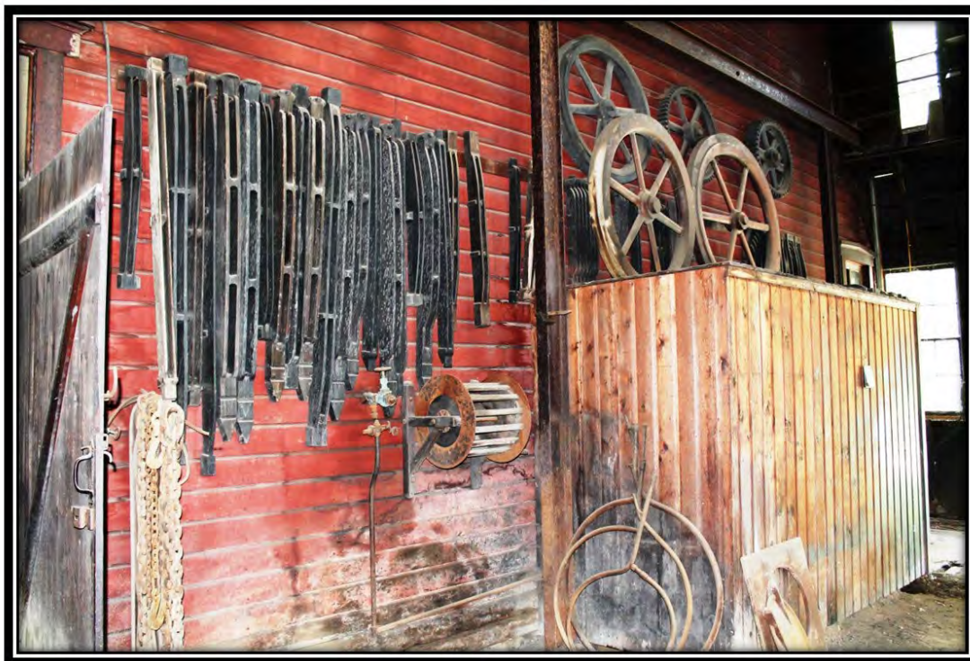
Photograph 34. PA_Greene County_W.A. Young & Sons Foundry and Machine Shop_0034. Patterns hanging on the west wall of the Foundry and the women's toilet, facing north. Note the Front Shop's clapboard-sided, former exterior wall.
