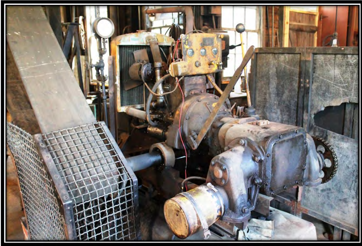
Photograph 14. PA_Greene County_W.A. Young & Sons Foundry and Machine Shop_0014. Former gasoline tractor engine and its transmission, with main belt to the line shaft that powers the shop, facing south.
