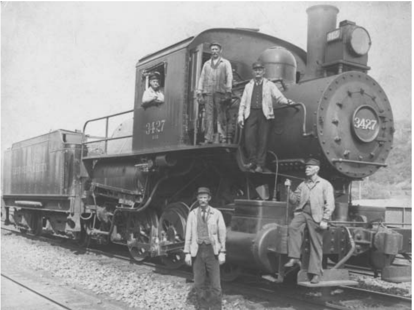
Camelback steam locomotives were used for local hauling around coal and rail yard operations.
