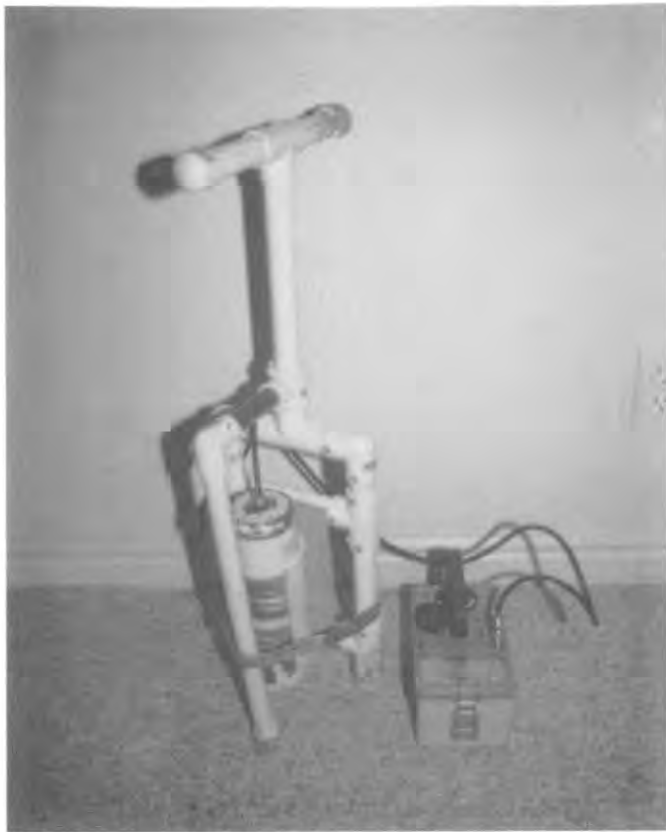
FIGURE 2 - Radiological survey instrument used to conduct the radiological survey at the theropod quarry Dinosaur National Monument. The instrument is an Eberline Micro-R meter with the scintillation detector mounted inside a lead shield.
