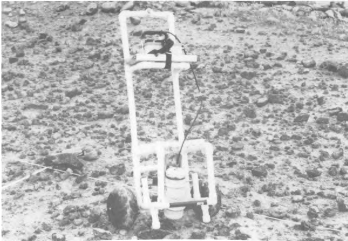
FIGURE 7 - Radiological survey instrument used to conduct the radiological survey at Hagerman Horse Quarry, Hagerman Fossil Beds National Monument. Instrument is an Eberline Micro-R meter with scintillation in a lead shield which is mounted on a cart.
