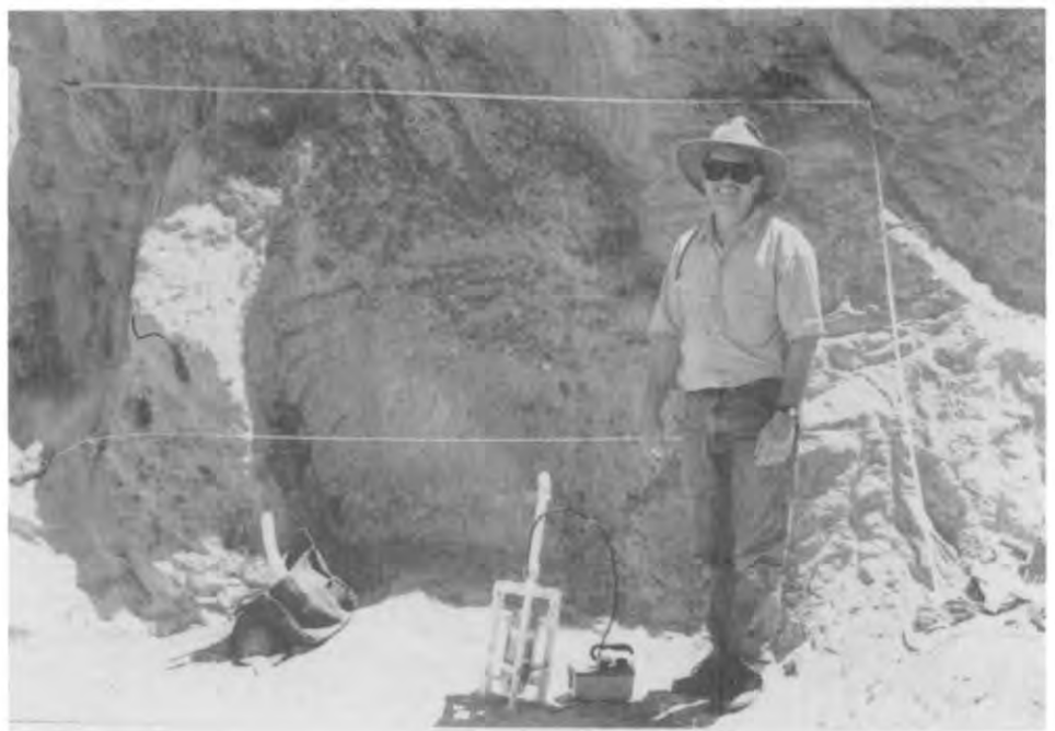
FIGURE 3 - Theropod Quarry, Dinosaur National Monument showing survey grid lay out, radiological survey instrument used to conduct the radiological survey, and Dan Chure, Paleontologist at Dinosaur National Monument.
