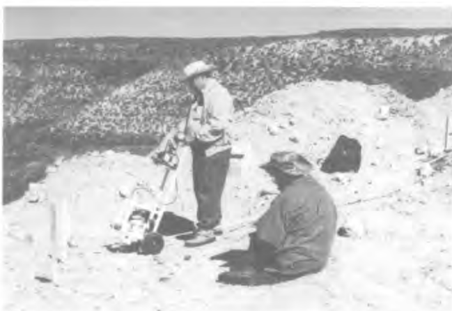
FIGURE 6 - Ramal and Carole Jones conducting the radiological survey at Hagerman Horse Quarry using the Eberline Micro-R meter with scintillation detector in a lead shield mounted on a cart. Carole Jones is recording survey data.
