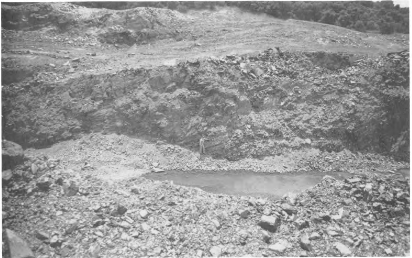
FIGURE 4 - View to southwest of quarry face at Clinton Block and Supply Site, Exposure includes base of gray thin-bedded shale at base on right, to top of thick-bedded red shale on left. Person is at contact of units. Dip of beds approximately 24°SE.
