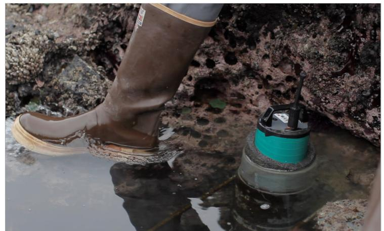
SeaFET™ pH sensors were incorporated into ongoing monitoring efforts at both NPS units.
