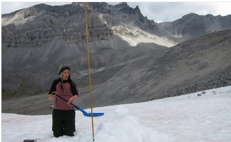
Tedesche digs a snow field test pit to look at layering of different phases/ages of snow and ice as they change over years of compaction, as well as measures temperatures to characterize the thermal gradient.
