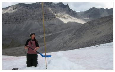
Tedesche digs a snow field test pit to look at layering of different phases/ ages of snow and ice as they change over years of compaction, as well as measures temperatures to characterize the thermal gradient.
