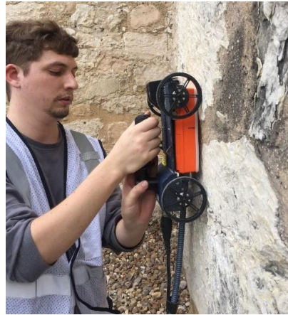
Figure 1.2a and b) Radar scanning on the interior of a historic stone masonry wall using a GSSI SIR-3000 radar unit with 1600 MHz antenna. Laser levels were used to guide the movement of the antenna on an accurate path and provide a consistent starting elevation for the vertical scans. (Author 2019)
