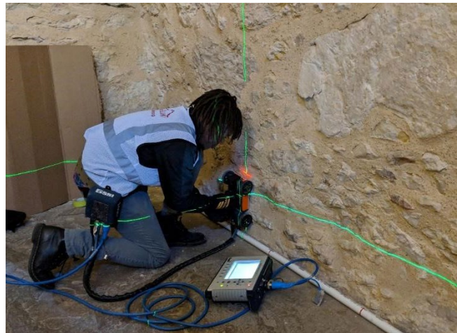
Figure 1.2a and b) Radar scanning on the interior of a historic stone masonry wall using a GSSI SIR-3000 radar unit with 1600 MHz antenna. Laser levels were used to guide the movement of the antenna on an accurate path and provide a consistent starting elevation for the vertical scans. (Author 2019)
