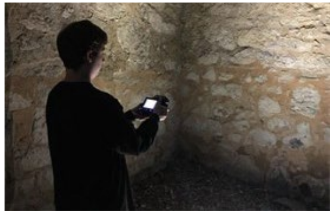
Figure 1.8 Recording a thermogram with an infrared camera. (Author 2019)
