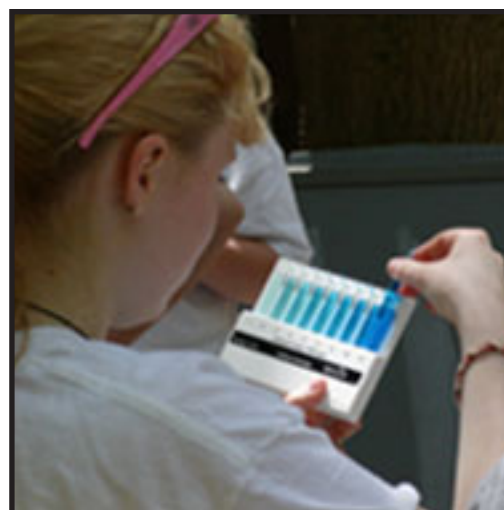
A student uses a simple water testing kit to determine dissolved oxygen content.
