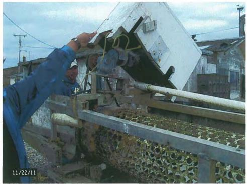
Photo 4. Oyster Tumbler Motor (and primary noise source)
