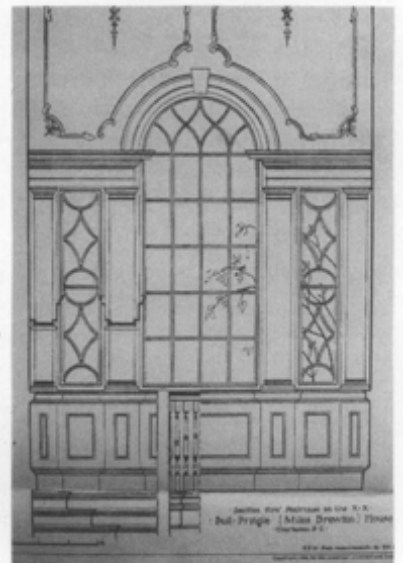
Figure 19. A drawing from the 1930s shows original ornament on the wall above a Palladian window in the 1760s Miles-Brewton House, Charleston, South Carolina. When the ornament was subsequently removed and lost, this scale drawing was used as documentation to fabricate matching ornament. Photo: Jonathan Thornton.
