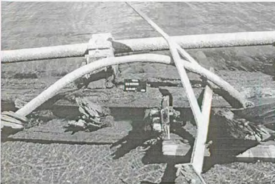
Figure 5.52. Davit (left) and support bracket (right) within E. C. Waters' wreckage. NPS photo by Brett Seymour.
