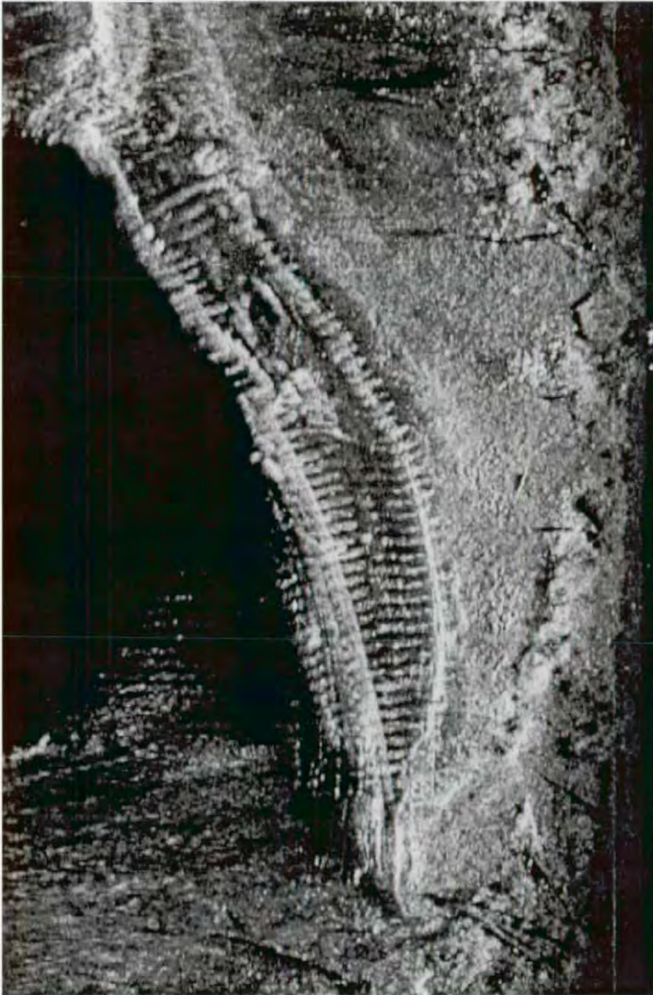
Figure 16. Sonograph of E. C. Waters' site showing hull features and surrounding bottom areas. Curvature is the result of the survey vessel's path. E. C. Waters' bow is at the bottom of the image.
