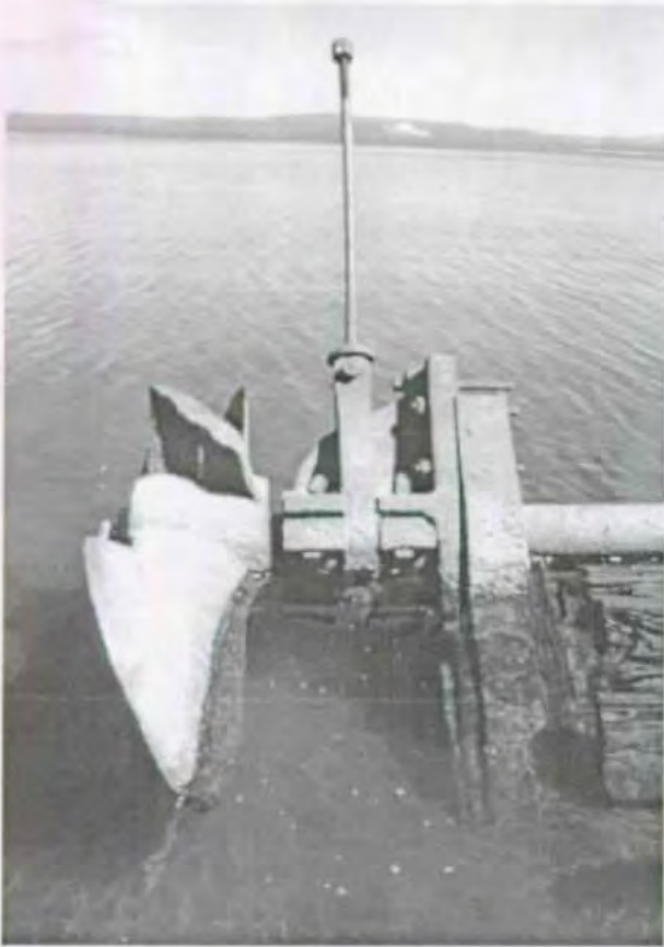
Figure 5.44. View north, starboard side of adjustable stern bearing assembly (center) and propeller (left). NPS photo by John Brooks.
