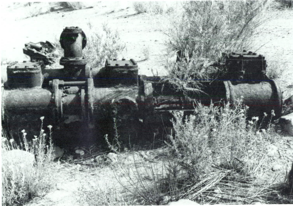
Figure 3.10. Closeup of the remains of one of Spencer's pumps used to convey water from the river to the hydraulic nozzles at the base of the cliffs. Photo by J. Bradford.
