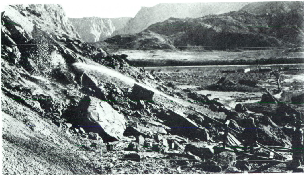
Figure 3.11. Hydraulic mining of the Chinle formation at Lee's Ferry in 1911. Water was pumped from the river, through the hose to the monitor or nozzle. The runoff was collected in a flume (right) and returned to the amalgamators at the river. Photo from Charles H. Spencer. Courtesy W. L. Rusko.
