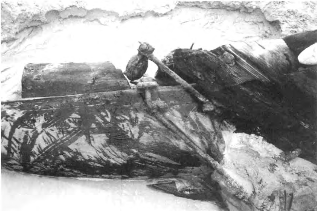
Figure 4.76. The port knighthead is the large timber on the right side of the photograph. The bowsprit extends horizontally to the left in the photo with the jibboom heel chock on top; also visible are the gammon iron and a single bull's-eye that held the foremast stay.
