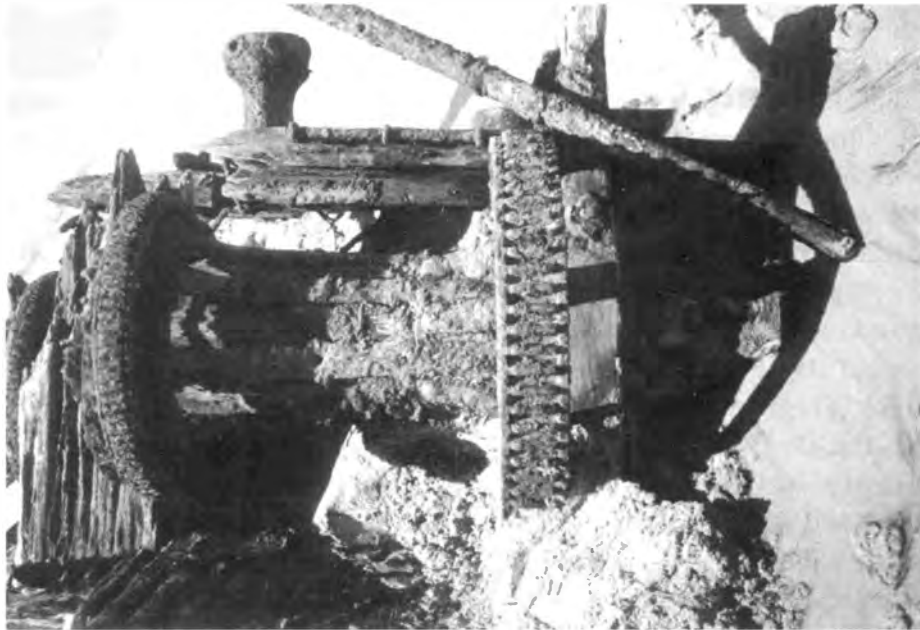
Figure 4.94. Comet's windlass mounted on the main deck. NPS photo by Matt Russell.
