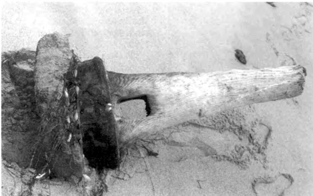
Figure 4.49. Portion of a rudder stock with the iron yoke that attached it to diamond-cut screw steering gear. NPS photo by Don Morris.
