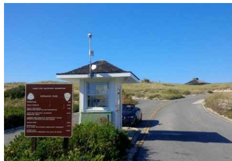
Cape Cod National Seashore uses camera-based, internet-enabled parking lot traffic counters (Photo credit: NPS).
