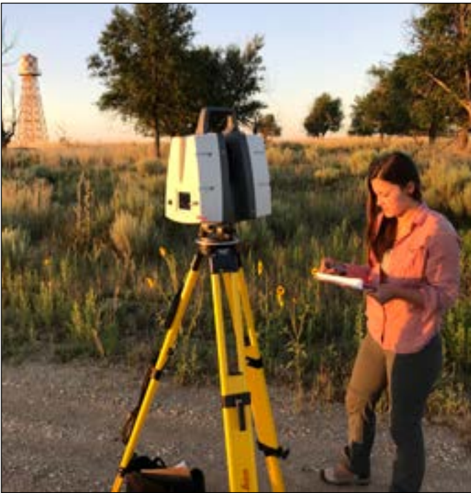
UC Denver uses LiDAR scanning technology to document existing and reconstructed buildings at the former Amache incarceration site. Photo courtesy of Michael Nulty, University of Colorado Denver.
