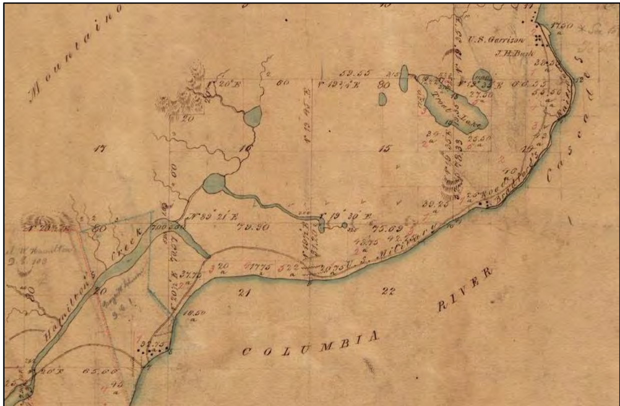
Figure 35. This General Land Office (GLO) map from an 1860 survey shows the northern bank of the Cascades portage. There is a U.S. Garrison (Fort Lugenbeel) at the beginning of the portage, with several structures nearby. “Bradford’s Railroad” is drawn along the shore, and further inland is the “U.S. Military Road” that followed the Chinookan portage route.
