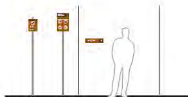
RR011 Regulatory Post Mount, Single Reg RR012 Regulatory Wall, Post, or Chain Mount RR013 Directional Wall Mount
