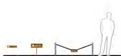
RR030 Low Profile Regulatory ground mounted RR031 Low Profile Regulatory moveable RR032 Low Profile Regulatory fence/chain mounted
