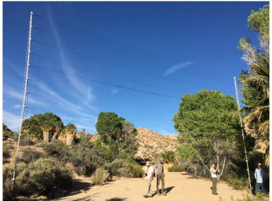
Figure 7. A mist net is set across a drainage downstream from a spring at Joshua Tree National Park. This type of set up is known as a “triple high” because it stacks three 3-meter tall nets on top of each other on poles with a pulley system that can raise or lower the nets.
