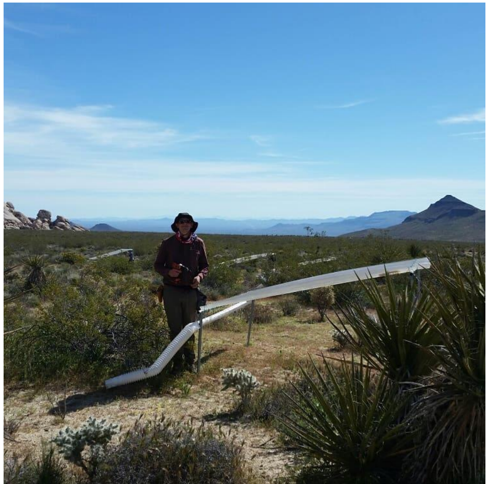
Figure 2. An example of a drought-inducing shelter that induces a 66% reduction in rain below the canopy. Notice the white tubing laying in front of Tim Ohlert, this drained the water that was captured in the v-shaped panels across the top. In the background you can see three more of the seven total drought-inducing shelters located at the East site within the Granite Mountains Desert Research Center.
