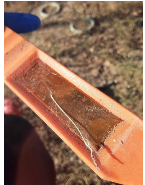
Figure 5. PRS® probe after ~4 months of deployment, with a plant root embedded in the ion exchange material. Probes were shipped to Western Ag Innovations where positive and negative ions (soil nutrients) were stripped from each resin membrane using a strong acid or base bath. Extracts were then analyzed for concentrations of 11 different soil nutrients: Mg, P, K, NH 4 , NO 3 , Cd, Ca, Al, Mn, Pb, and Fe.
