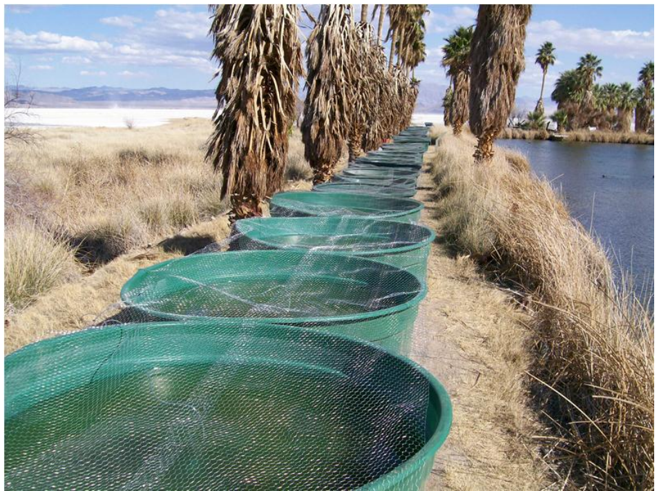
Figure 3. Thirty 320 gallon plastic cattle tanks were used for the field mesocosm experiment. Mesocosms are a good way to study species interactions under semi-natural conditions. Each mesocosm was filled with Lake Tuendae water, provided with 3 m of plastic “plant” material, and covered with poultry fence to avoid fish suicidal jumps and bird predation. Lake Tuendae is visible to the right and Soda Dry Lake can be seen in the background. Photo: Sujan Henkanaththegedara ©.
