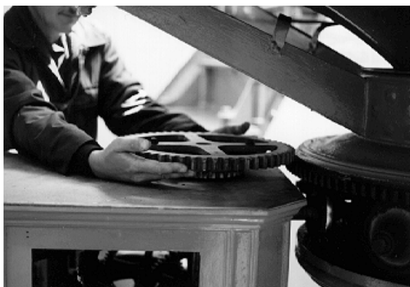
Figure 34. When this first-order classical lens was converted to AC power, the original drive gear (pictured here) was the crank used to wind the clockworks.
