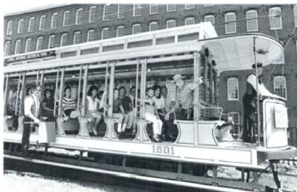
The first streetcar built for the Lowell Park Trolley system was based on a 1901 Brill car that ran in Lowell at the turn of the century.
