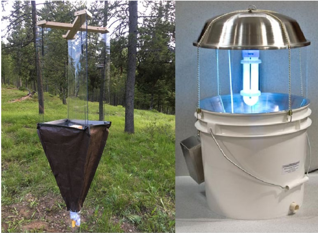
Figure 2.2. Insect trap designs. Flight intercept traps (left) consisted of two 24"x18" acrylic sheets cut half way up their longitudinal axis and slid together, a wooden top support, and a tarp funnel below with a collection container. Collection containers were filled with cut pieces of No-pest® Strip2. UV bucket traps (right) use a UV bulb to attract insects toward intersecting acrylic sheets that stand above a collection container with No-pest® Strip2.
