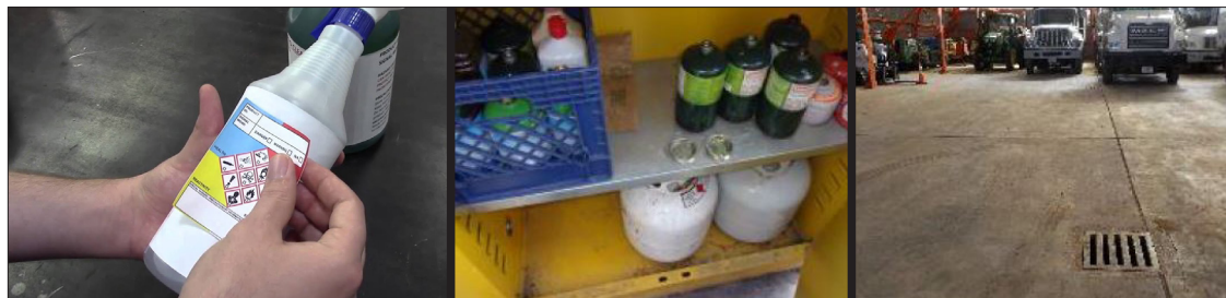
Environmental auditors want to ensure that Globally Harmonized System (GHS) labels are on secondary chemical containers, flammable materials are kept in flammable lockers, and that proper spill containment is in place
