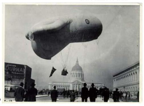
shape) consisted of a hydrogen-filled body equipped with fins that provided stability in rough air, and a suspended wicker basket that held a two-man crew. Communication between the observers and the ground crew was via a telephone cable spliced onto the mooring line. Before long, the Americans began manufacturing their own version of the French balloons, which the army designated the Type C-3. During 19181919, nearly a thousand C-3s were manufactured in the U.S.
