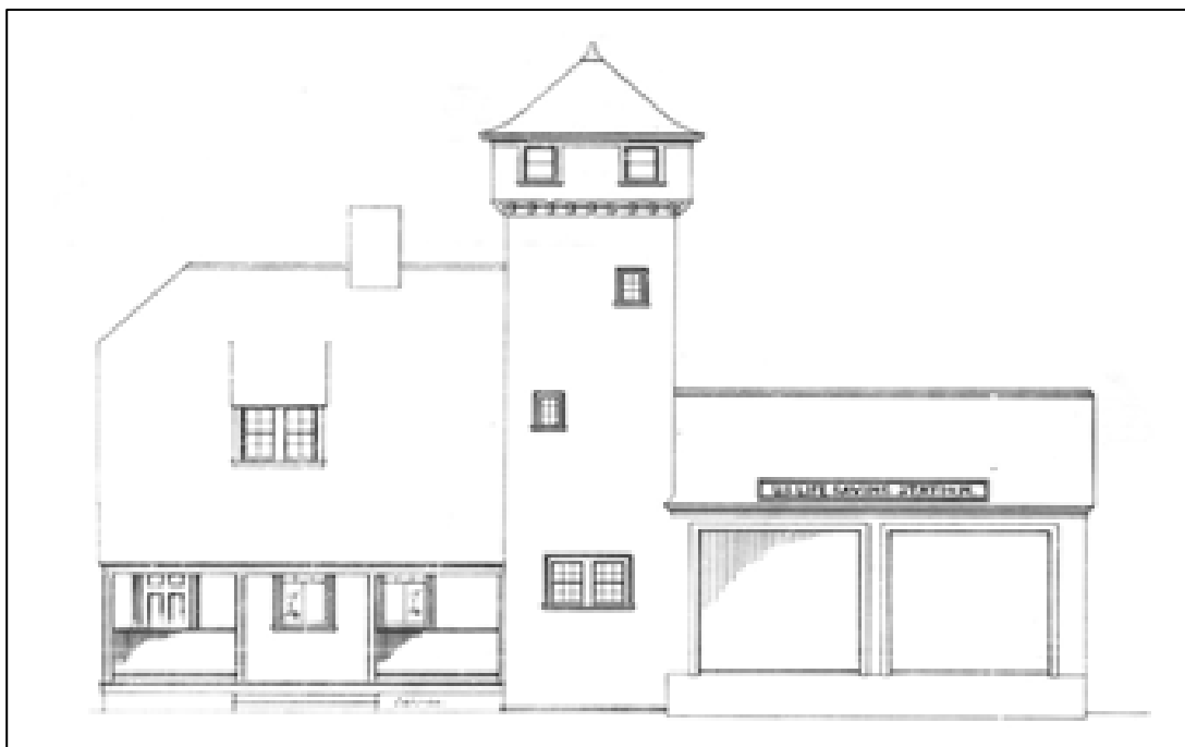
Figure 9. Front elevation of the Duluth-type life-saving station, designed by George R. Tolman (not to scale).
