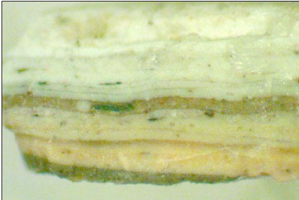
Figure 65. Spermaceti Cove Life-Saving Station, sample P087 taken from the East/Front Porch original northeast half-post.
