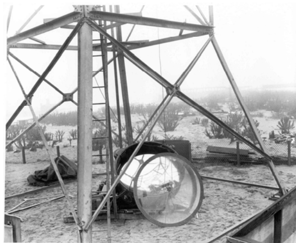
Searchlight tower in Sea Bright after the cable snapped and the light fell.
