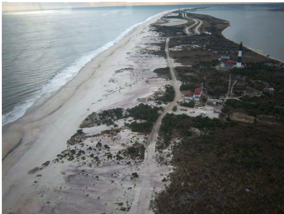
Photo 4: Post-Sandy view of lighthouse area looking west. NPS photo, 2012. Note the overwash areas, now flat, where dunes previously stood. The park entrance is just below the end of the divided roadway at the top of this photograph.
