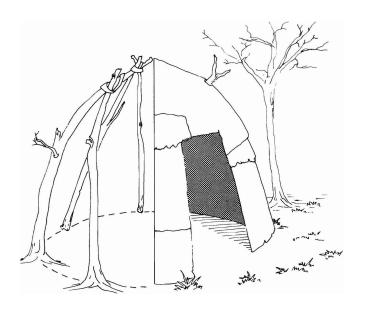
Figure 5. Big Bear-Holt wickiup along Paint Creek in first valley north of Waukon Junction. Small trees were bent over to form a round roofed wickiup covered with elm bark and sheet tin. Cutaway view. (Artist's conception by Demetrios Betinis, Field Museum of Natural History.)
