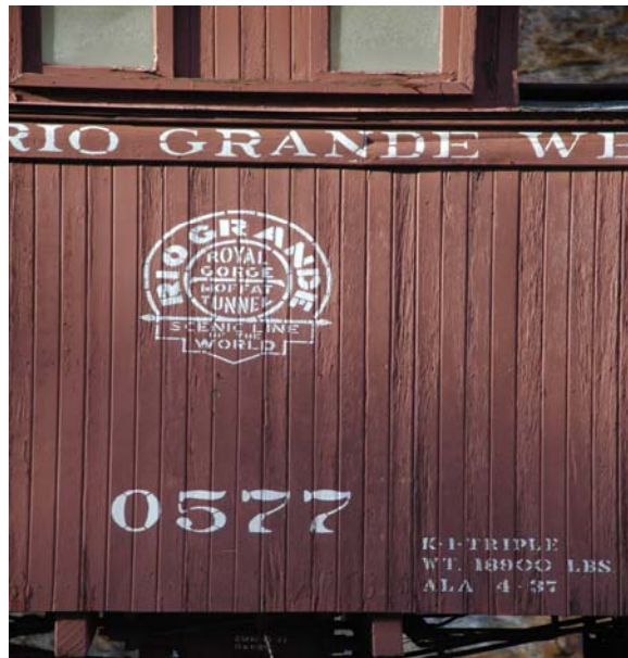
Figure 101. Wood Rot and paint peeling and bubbling on the right side
