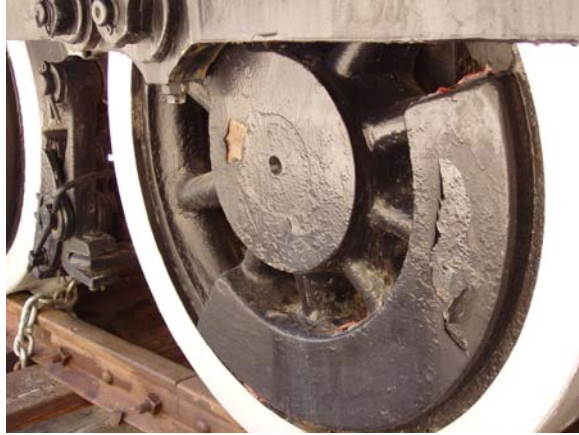
Figure 82. Rust and paint peeling on wheels
