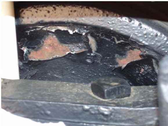
Figure 81. Rust and paint peeling on wheels
