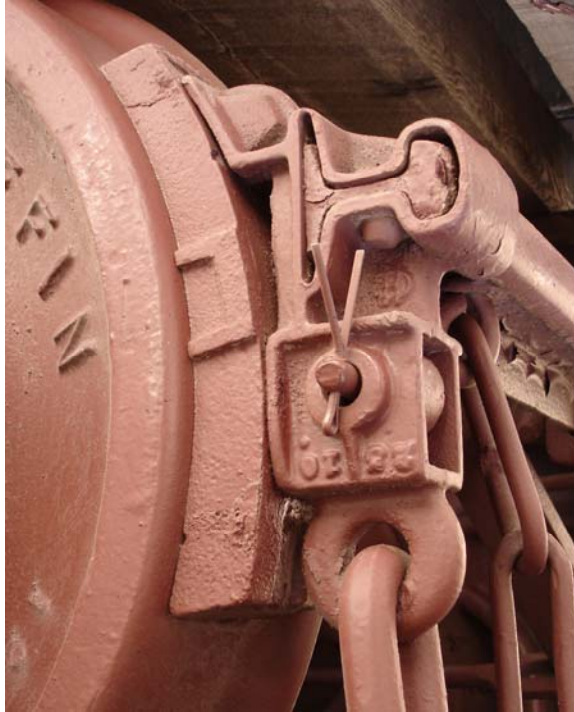
Figure 94. Brake beam and shoe are in good shape
