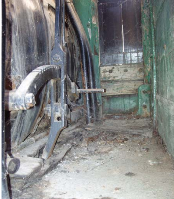
Figure 67. Dirt and animal droppings in the engineer's cab
