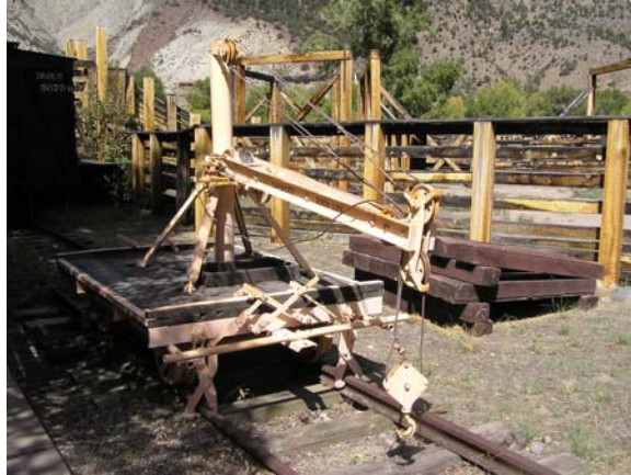
Figure 127. Crane car and aberration of steel wire
