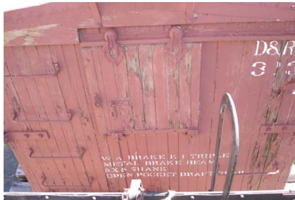
Figure 86. A end, sidings are weathered
