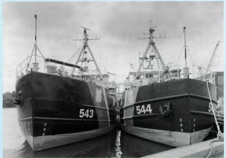
Two moored buoy tenders at the Coast Guard Yard at Curtis Bay in Maryland, White Holly on the left and White Sage on the right. The black hulls are a way for the Coast Guard to designate the functional and utilitarian nature of its fleet that tends to lighthouses, buoys, gongs, bells, whistles, and most all maritime navigational devices. Note the different hull construction built around the same shape but probably reflecting construction in different shipyards.
