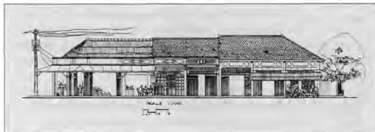
Measured drawings: Student-drawn elevation of shophouses in Chbar Ampau, Cambodia.
