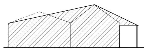
**Figure 17** Side elevation of Lewis-Davis House illustrating changes to roof line after WWII. (T. Jones, NPS-SERO-CR, 2002)
