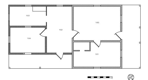
**Figure 14** Reconstructed floor plan of house as it was constructed in the 1920s. (T. Jones, NPS-SERO-CR, 2002)
