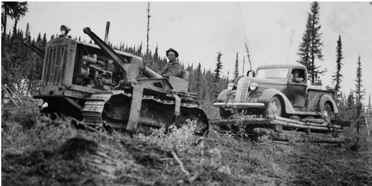
A Caterpillar "Diesel Forty" pulling a Dodge truck on skids to Coal Creek mining camp, ca. 1936. University of Alaska Fairbanks, Stanton Patty Family Papers (2012-93-80).
