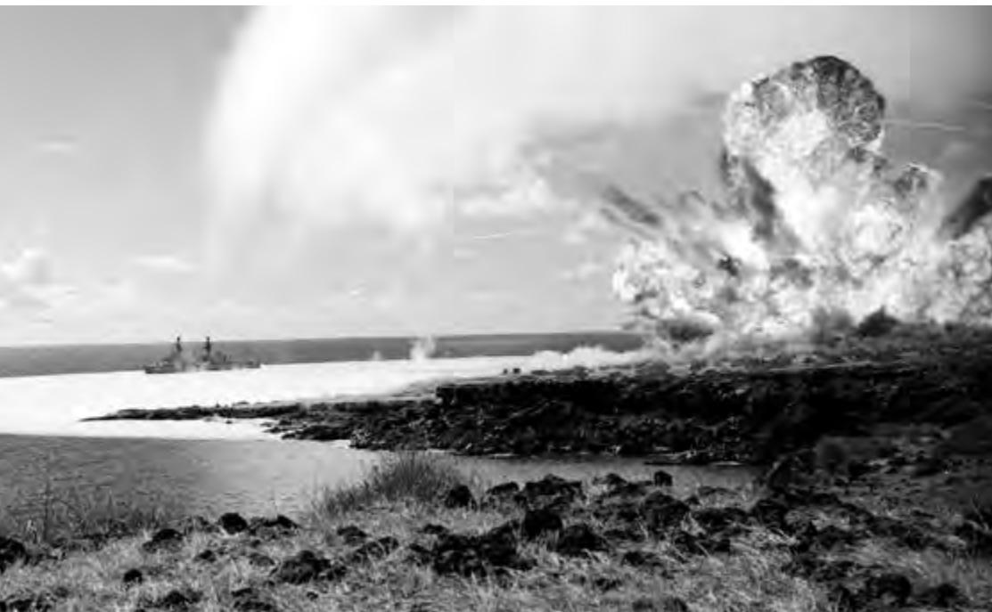
The detonation of a 500-ton TNT explosive for Shot Bravo, the first of three test explosions in Operation "Sailor Hat" on Kaho'olawe, was meant to simulate the effects of nuclear bombs on naval vessels anchored off shore. It is believed to have cracked the island's water table.
