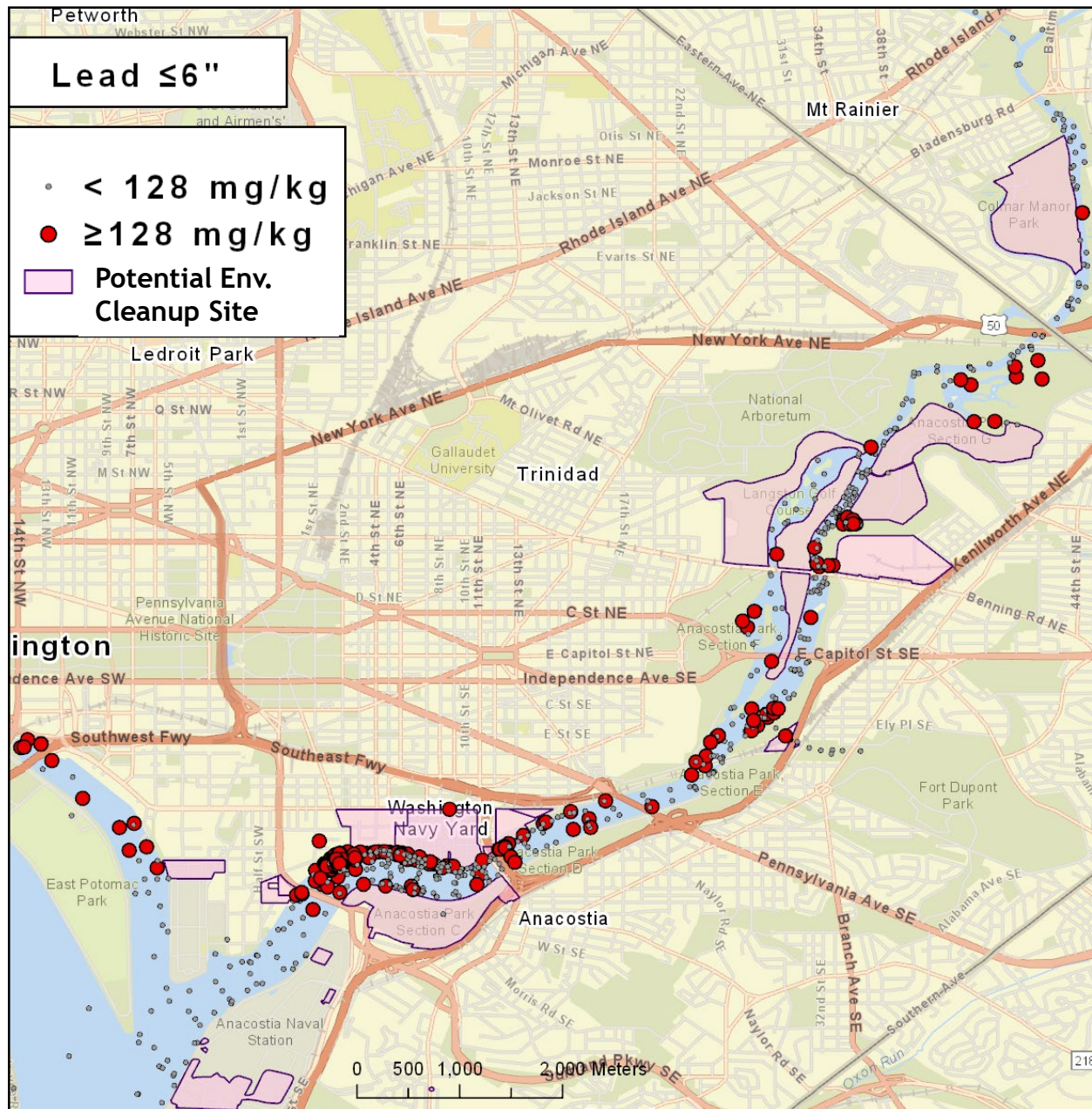
Figure 5. Lead concentrations in surface sediment samples collected from the tidal Anacostia River between 1989-2016 compared to the consensus-based probable effect concentration, 128 mg/kg (below =grey; exceeded =red). Outlines of potential environmental cleanup sites are also indicated.
