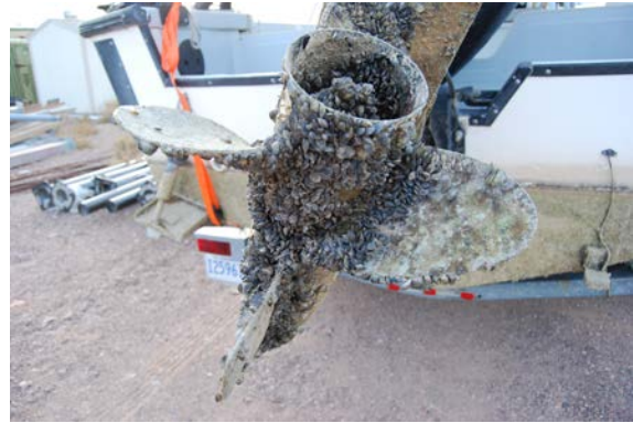
Boat damage due to the aquatic invasive quagga mussel.
