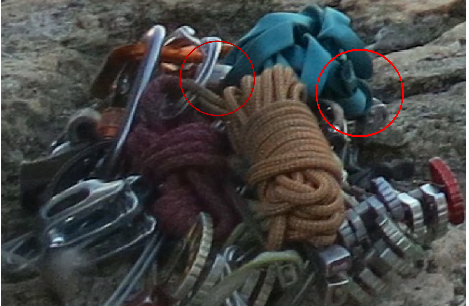
Previous Photo Zoomed In: The Water Knot in the blue 9/16 Tubular Webbing is not tight. The knot's "bottom" tail is visible. The webbing is configured to carry cordellette style. The locking mechanism on the carabiner that is attached to the webbing appears to match the free locking carabiner that was found on the anchor post fall.
