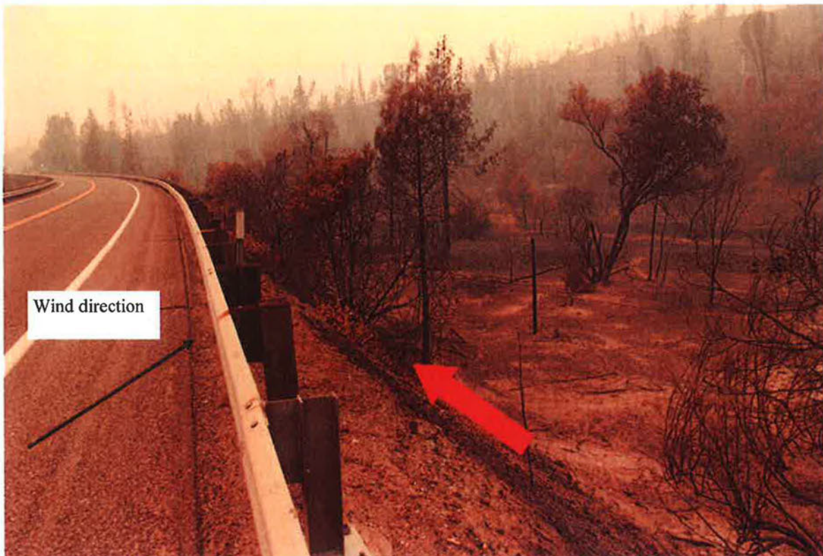
Photo 9—IMG_0764 West Vegetation with angle of char. Area not affected by reburn. Fire advanced up slope and then wind bent flames back to create angle of char.
