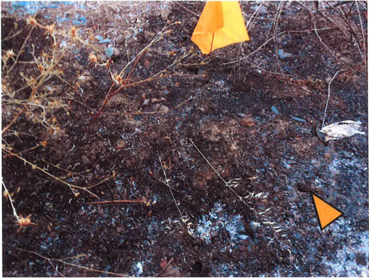
DSCN0830- Photo 14 (Fire B) Grass stem fire pattern indicators. Right lateral fire vector with low intensity fire
