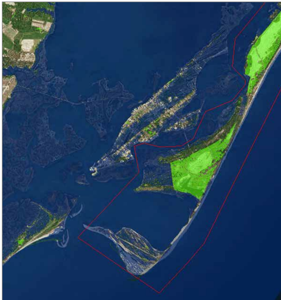
Figure 2. An example of how areas of inundation appear in ArcGIS. In this example for the Toms Cove area of Assateague Island National Seashore, areas of inundation (RCP4.5 2050) appear in blue. Green shading indicates other low lying areas that are blocked from inundation by some impediment, but nonetheless could experience flooding should the physical barrier be removed or breached.
