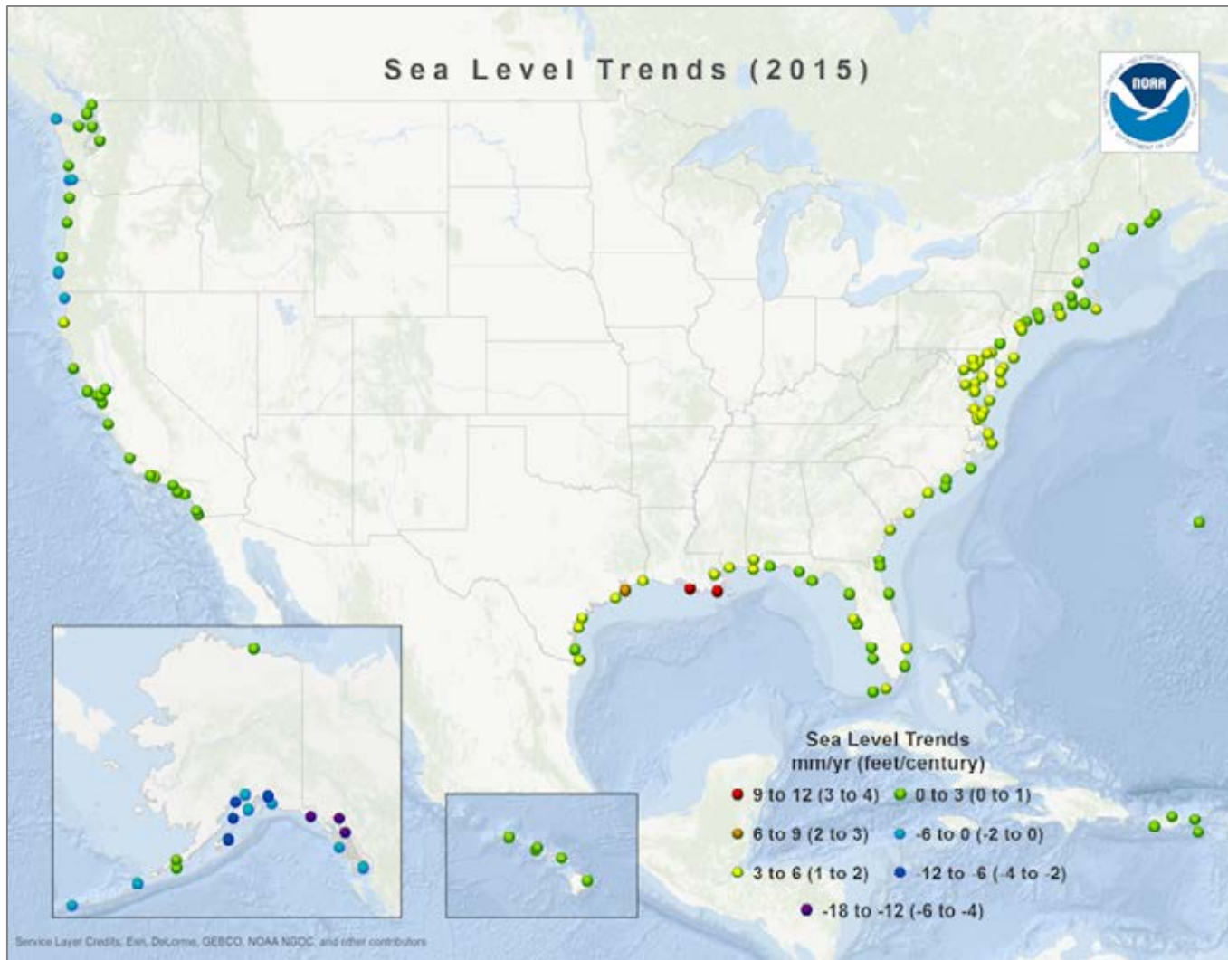
Figure 1. Sea level trends for the United States based on Zervas (2009), for all available data through 2015. Each dot represents the location of a long-term (>30 years) tide gauge station. Green dots represent stations that are experiencing the average global rate of sea level change. Stations depicted by yellow to red dots are experiencing greater than the global average (primarily driven by regional subsidence) and blue to purple dots are stations experiencing less than the global average (due to isostatic rebound or other tectonically-driven factors). Source: https://tidesandcurrents.noaa.gov/sltrends/slrmap.htm
