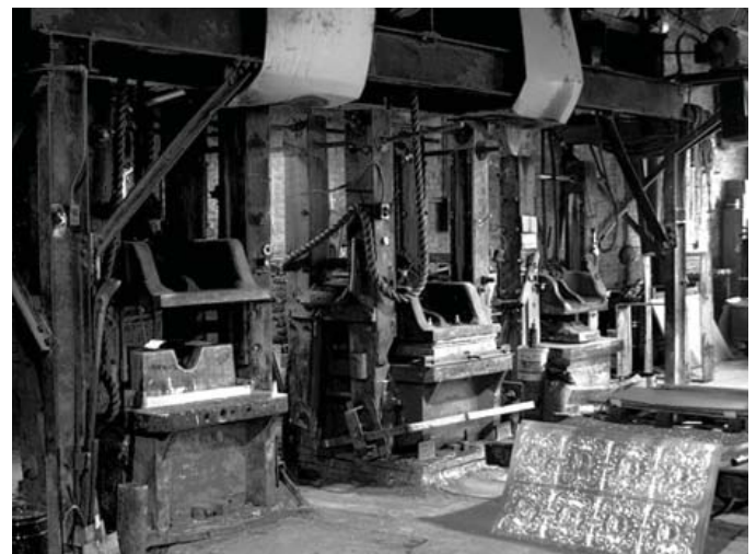
Rope drop hammers at the turn-of-the-century factory in Nevada, Missouri, that W. F. Norman Corporation still uses to stamp individual panels, resulting in high quality pressed metal sheets. (Photo: W. F. Norman Corporation)
