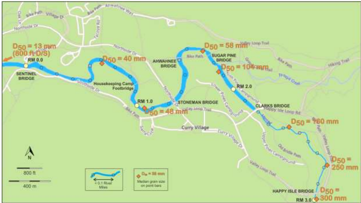
Figure 3-8. Median grain diameters ( D_{50} ), measured on the upstream low-water margin of point bars or mid-channel bars, sites where the clasts are most likely to reflect the active bedload during transport events (Kondolf et al. 2003). Note the progressive, monotonic decline in median size, with particularly rapid changes where the river emerges from confining bedrock and talus fields downstream of Happy Isles Bridge, and as it passes through the short reach that includes Sugar Pine Bridge.
