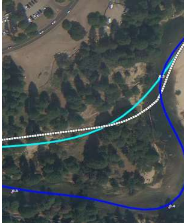
Figure 5-16. Cutoff and migration at RM 0.3 to 0.5. White dashed line shows the path of the most probable cutoff; light blue line indicates the centerline of subsequent migration.
