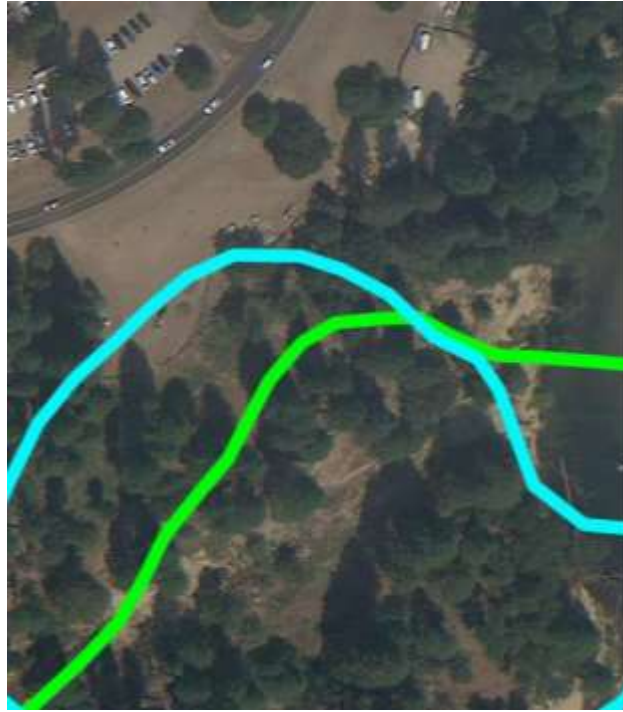
Figure 5-2. Historical progressive migration 1870-1883 at RM 0.3 to 0.4. The channel migrated from green to blue.
