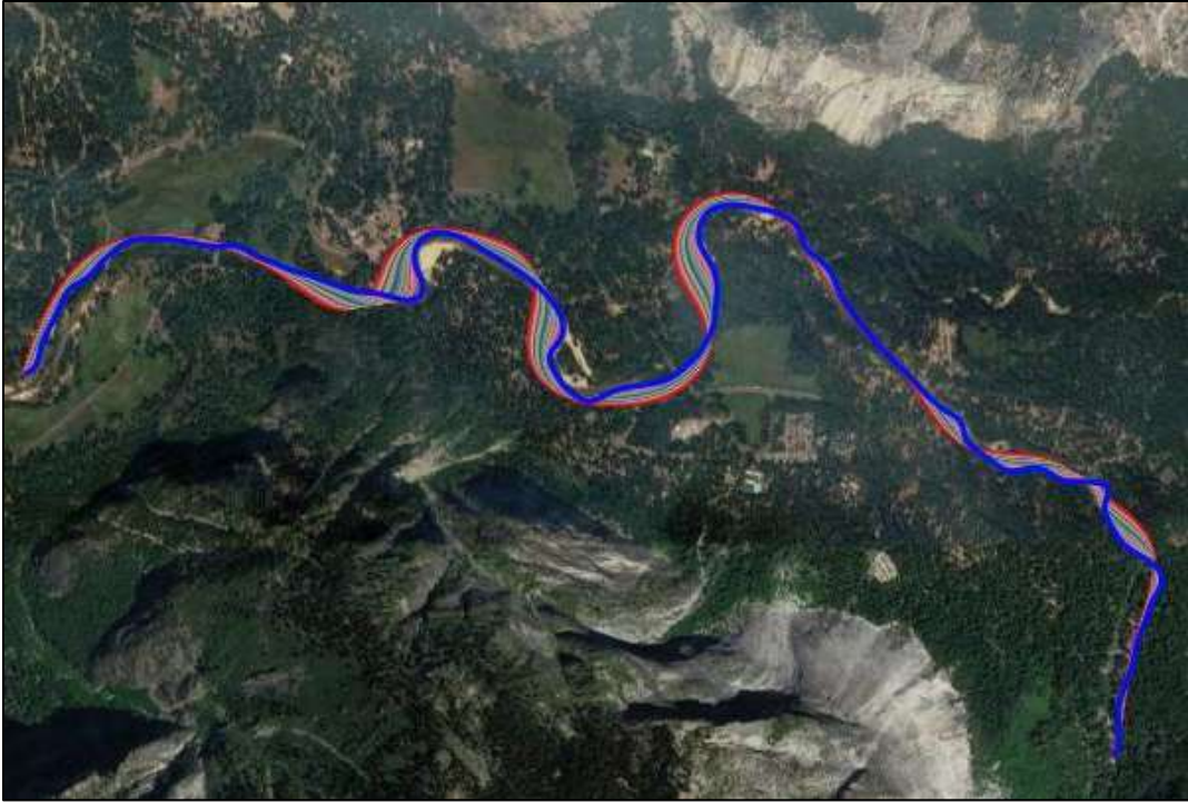
Figure 5-5. Channel migration 2016 to 2067 without revetments in place. The blue line represents the channel centerline in 2016; the red line represents the channel centerline in 2067 modeled with no revetments.
