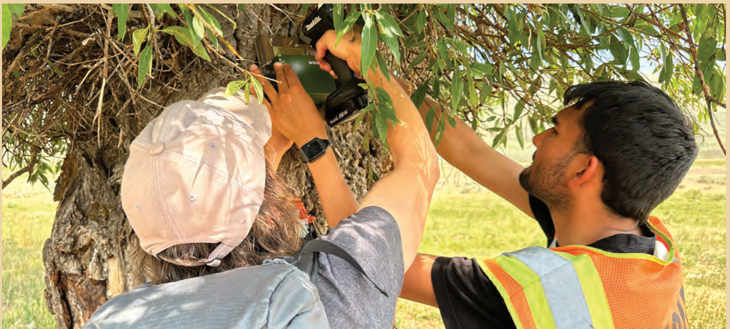
Jeff Reed of Grizzly Systems Inc (left) and Jeremy SunderRaj attach one of the autonomous recording units to a tree. This unit will collect audio data for at least 30 days, 24 hours each day and provide valuable information on all vocal wildlife species and human-generated noise in Yellowstone's northern landscapes. NPS Photo/ T. Rabe
