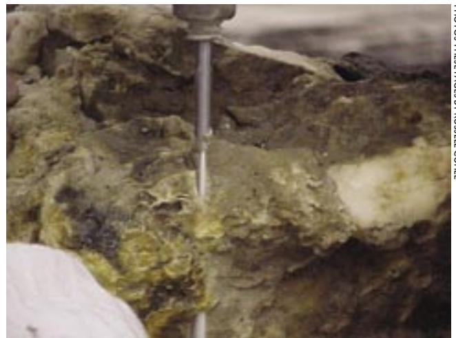
Figure 5. The water-jet saw finishes a transverse section across the bottom of the spire with the nozzle held close to the surface of the object.
