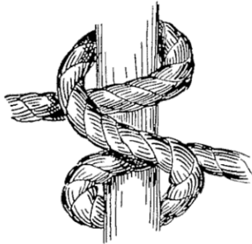
FIG. 36 A.—Clove hitch or builder's hitch (tying).
