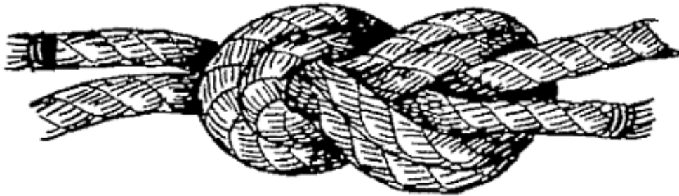
FIG. 24.—Double figure-eight knot (complete).
