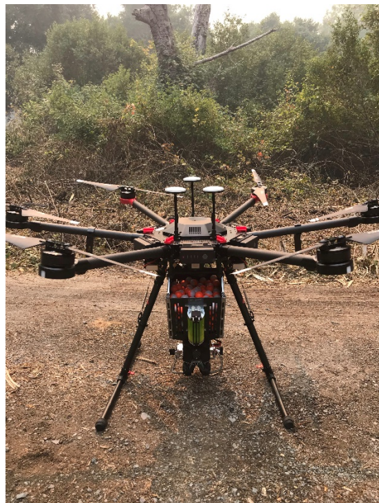
Drone equipped with PSDs— used for tactical firing operations.
