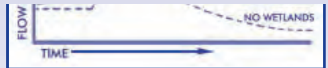
This diagram indicates that wetlands reduce peak stormwater flows. (Source: Kusler 1983)
