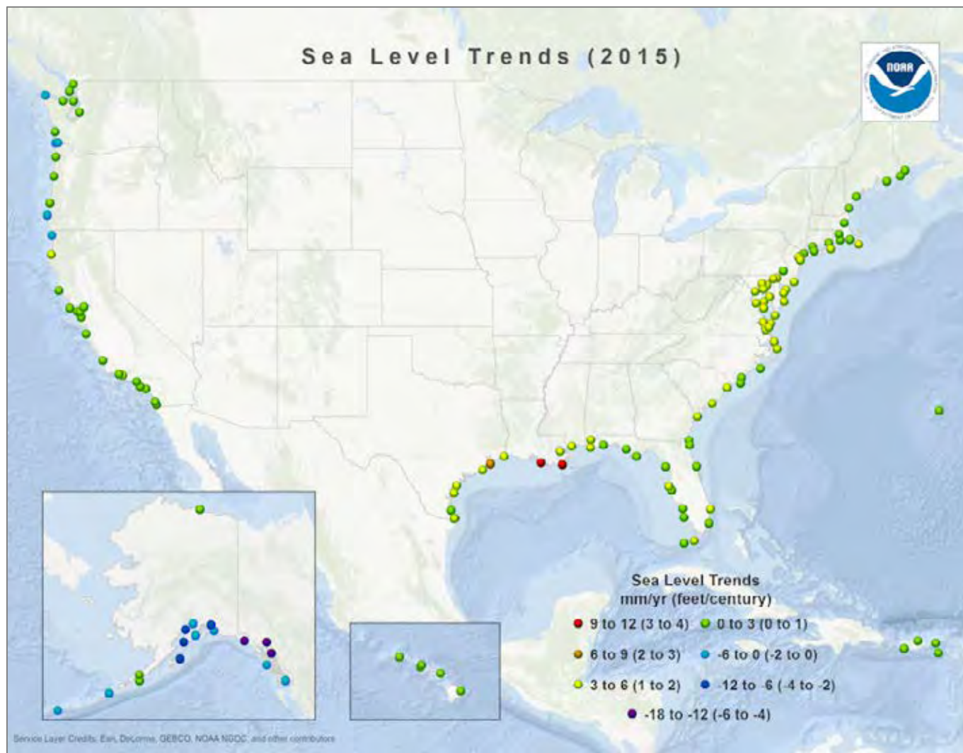
Figure 1. Map of the United States showing Sea Level Trends (2015) with color-coded dots indicating the rate of sea level rise in mm/yr (feet/century). The map includes insets for Alaska and Hawaii. A NOAA logo is in the top right corner.
