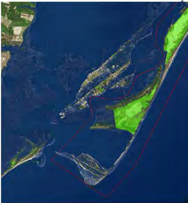
Figure 2. An example of how areas of inundation appear in ArcGIS. In this example for the Toms Cove area of Assateague National Seashore, areas of inundation (RCP4.5 2050) are shown in blue. Other low lying areas that are blocked from inundation by some impediment are shown in green.
