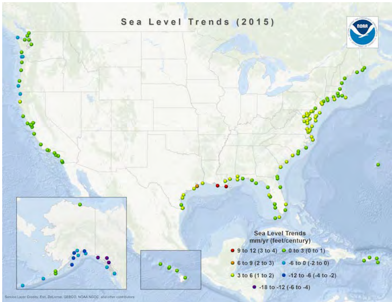
Figure 1. Sea level trends for the United States based on Zervas (2009). Trends are calculated for 2015 relative to global mean sea level. Each dot represents the location of a long-term (>30 years) tide gauge station. Green dots represent stations that are experiencing the average global rate of sea level change.
