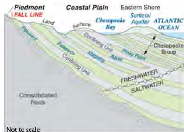
Figure 5.4. Schematic cross-section of the Coastal Plain aquifer system. 33
